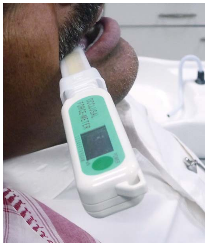
Fig. 1. Measuring bite force using a force transducer occlusal force meter (GM10; Nagano Keiki).
