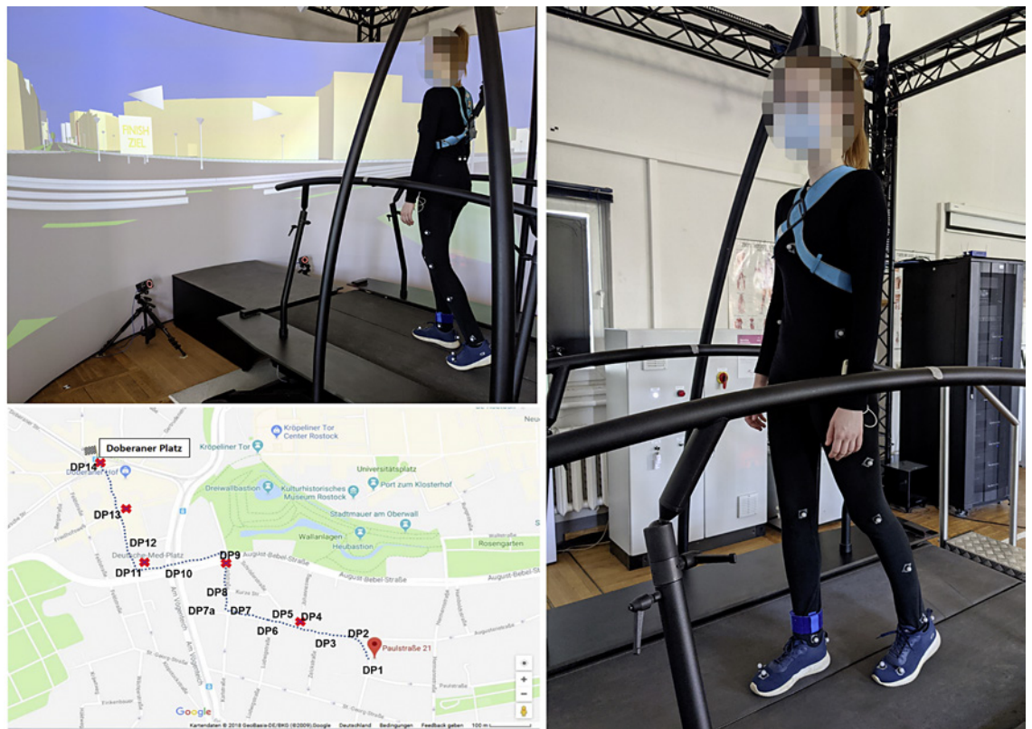
Fig. 1. Depiction of the experimental setup (top left and right). Image is used with permission of the participant. Wayfinding route (bottom left). Red crosses denote locations where the VE was manipulated in the experimental group. DP1 to DP14 indicate the DPs from start to finish. The changes as described earlier were always the same for all older participants in the experimental group.
